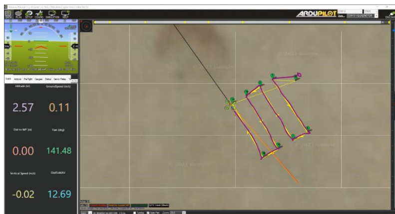
Figure 12. Flying the drone in a zig-zag trajectory at an altitude of around 2.5 m
